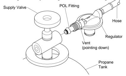
Figure 2 - Regulator With Vent Pointing Down
